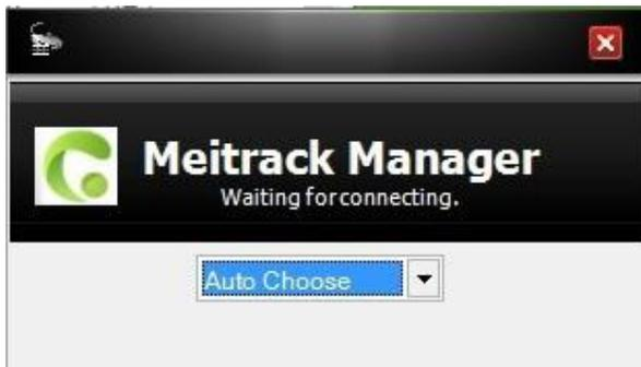
Turn on the device, then Meitrack Manager will detect the device model automatically and the parameter page will appear accordingly.
