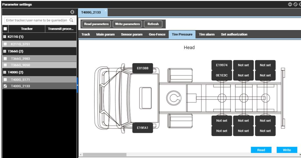
As shown in the above figure, the third tire on the vehicle's head part is bound to the tire pressure sensor whose ID number is E19974, and the fourth tire is bound to the tire pressure sensor whose ID number is OE1E3C. After the tires on the vehicle's head part are bound, you can move the horizontal scroll bar to bind the tires of four trailers.
