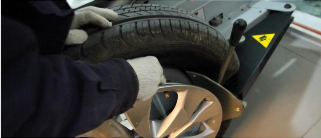
(4) Install and fasten the sensor tail and valve stem.
