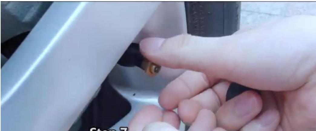
(3) Install the external tire pressure sensor.
