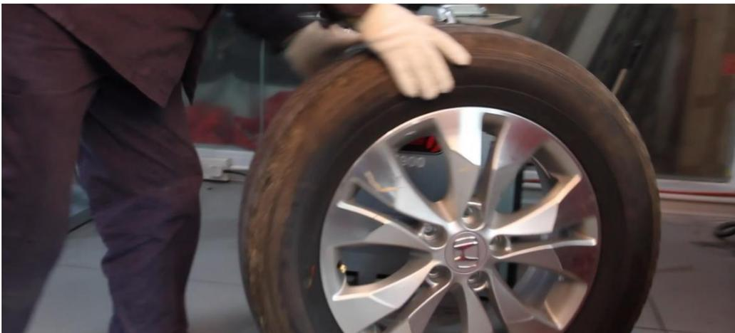
(3) Remove the tire from the wheel rim and shovel the original tire valve.
