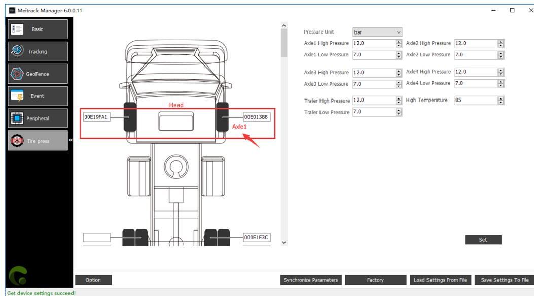
Use a large vehicle as an example. As shown in the above figure, bind the first tire on the vehicle's head part to the tire pressure sensor whose ID number is E01388, and bind the second tire to the tire pressure sensor whose ID number is E19FA1. In addition, set the high pressure thresholds of 4 axles and the trailer to 12 bar, the low pressure thresholds of 4 axles and the trailer to 7 bar and the high temperature threshold to 85°C.
