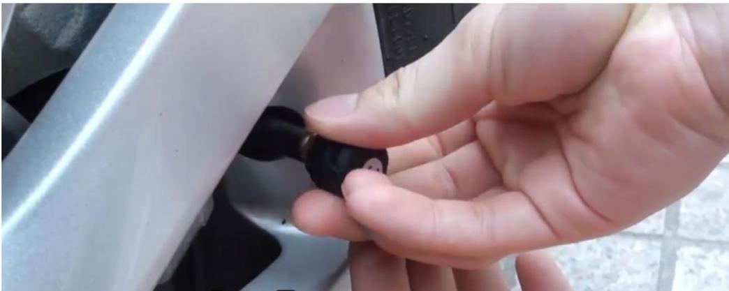
(4) Fasten the lock nut anticlockwise by clamp to prevent sensor theft.
