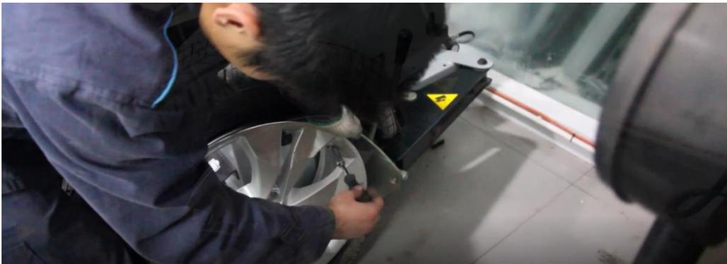
As shown in the following figure, the sensor tail is installed inwards, the valve stem is installed outwards, and the nut is fastened.
