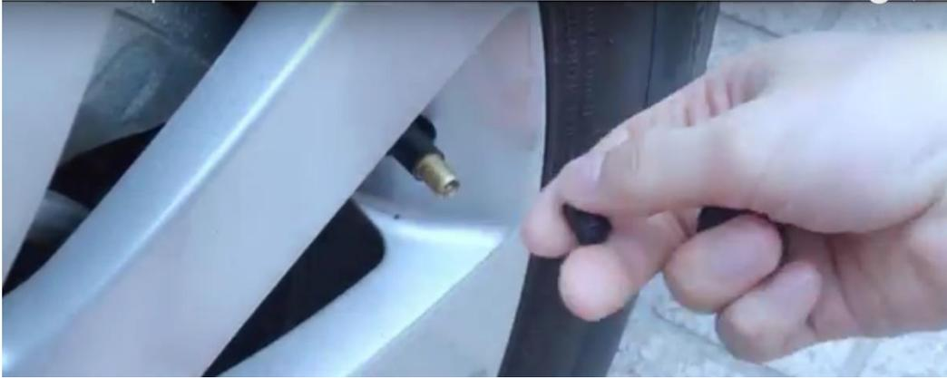
(2) Screw the lock nut onto the valve stem.
